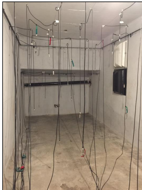
Figure 2: Test room interior. 20 Matched measurement microphones were uniformly distributed in the space, and hung vertically at different heights. On the right wall two samples of the acoustic diffusers are shown.
