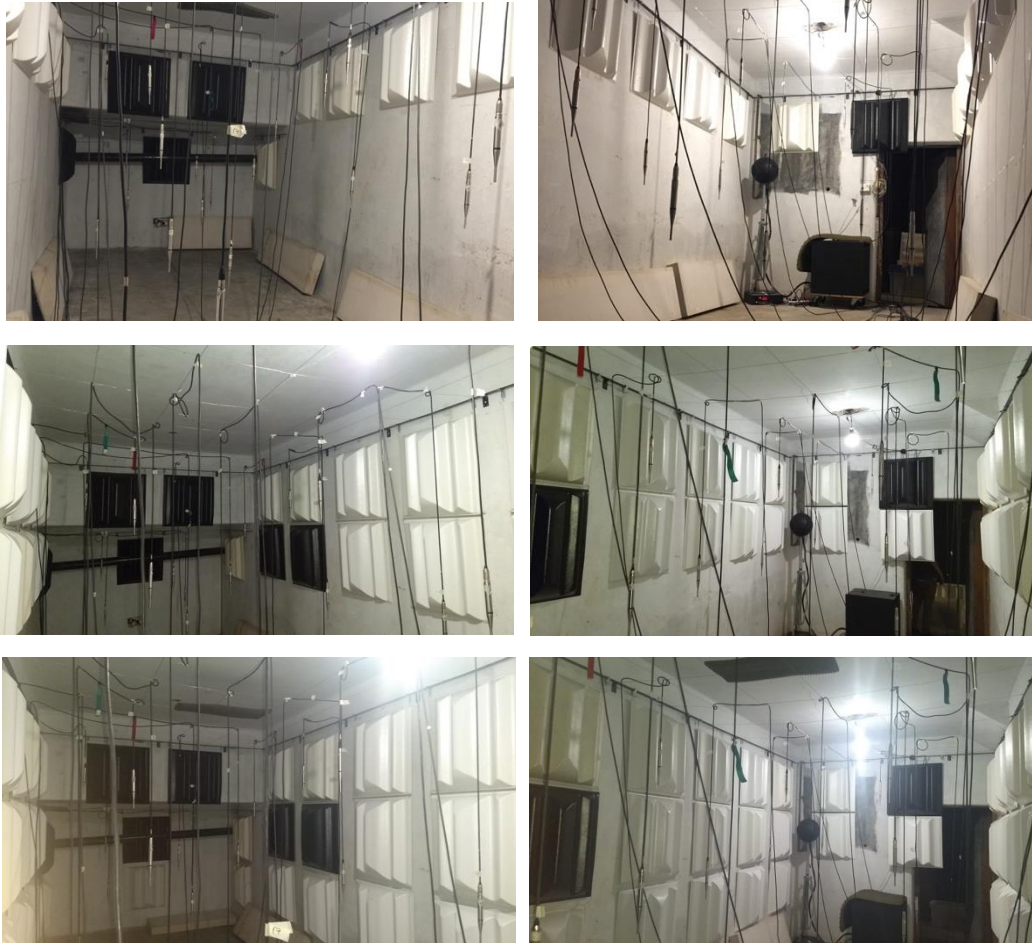
Figure 3: Pictures of test room with the diffusers uniform distribution configurations for three different coating surface extensions. At the bottom of the room can be seen the full band absorbers to set different reverberation and early decay times. At one dihedral corner, the omnidirectional sound source (mounted on a rotating turntable) and subwoofer (not used) can be seen. Upper paired pictures: one row uniform distribution configuration. Mid paired pictures: two rows uniform distribution configuration. Lower paired pictures: three rows uniform distribution configuration.
