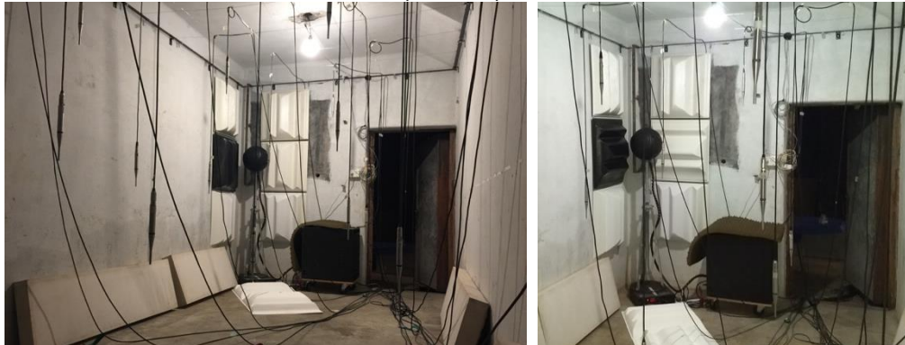
Figure 3: Test room with the diffusers concentrated distribution configuration around the sound source. At the sides of the room can be seen the full band absorbers to set different reverberation and early decay times. At one dihedral corner, the omnidirectional sound source (mounted on a rotating turntable) and subwoofer (not used) can be seen.
